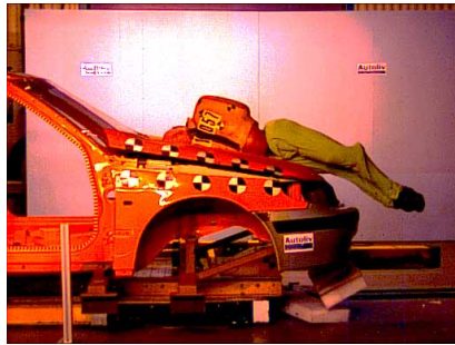
Figure 10. Crash test in 40 km/h with a pedestrian dummy and an active bonnet.
