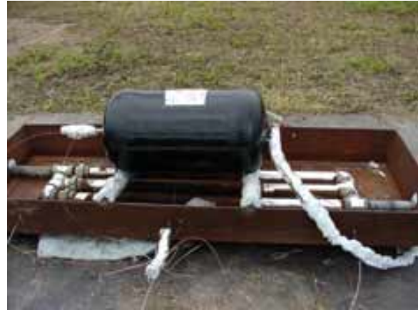
Figure 3. Hydrogen Fuel Tank in Bonfire Test Fixture
