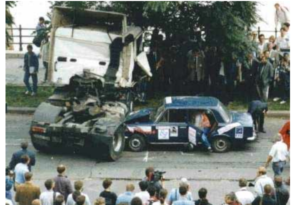
Figure 12. Real truck-automobile side impact reconstruction test.
