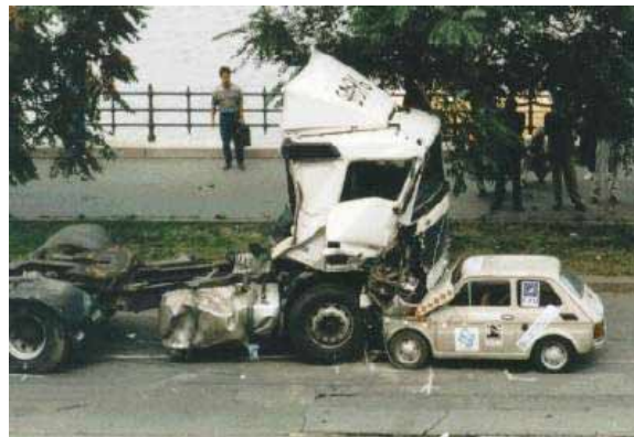
Figure 10. Front underrun accident reconstruction of small automobile with truck.
