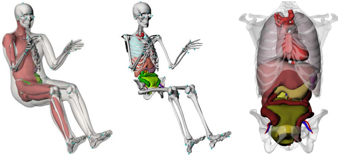
Figure 4. Assembled 3D F05 Occupant. Images show the full skeleton and all internal organs that will be explicitly represented. Bony landmark data is shown as blue points.
