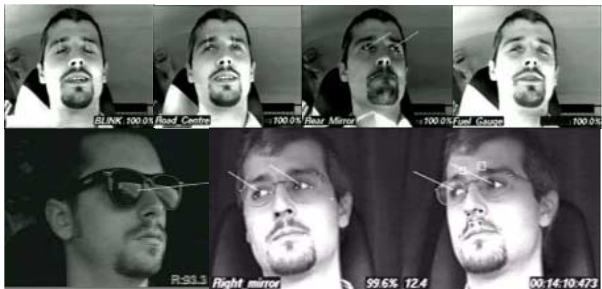
Figure 1. Images from the Volvo/ANU head and gaze-tracking system. The two images on the bottom right illustrate the output from the stereo cameras, with the tracking templates shown as boxes and reference points as white dots. The top row shows images taken in a Volvo V70 car and the bottom row shows images from a Volvo FH12 truck.
