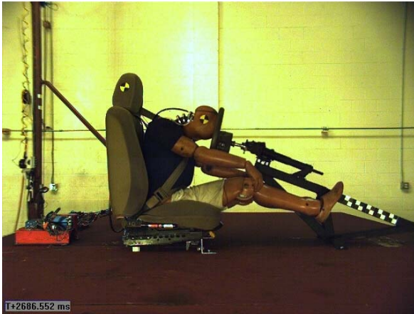
Figure 6. Hybrid III dummy with reduced musculature neck.
