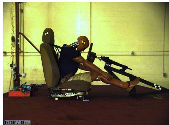
Figure 5. Hybrid III dummy with original musculature neck.
