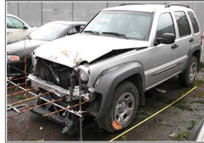
Figure 1. Photograph of Vehicle Being Measured for Crush Damage.
