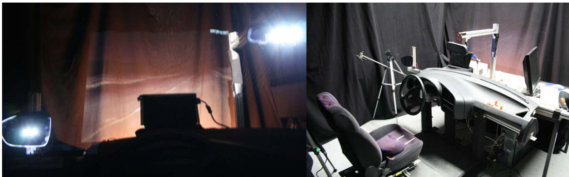
Figure 20: Experimental set-up for determining rear glare
