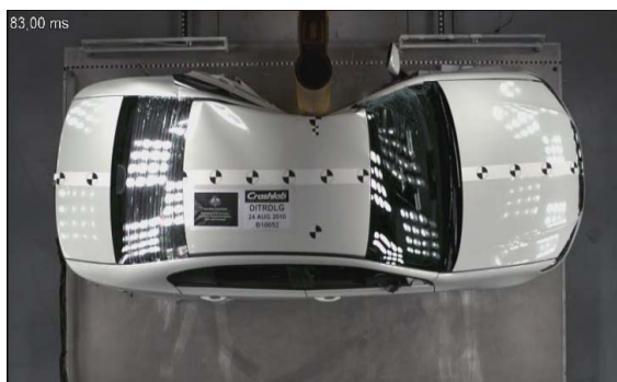
Figure 5. Australian Pole Side Impact Testing
