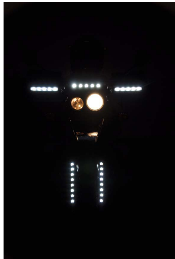
Figure 18: T-Design for nighttime, daytime running lights are used as position lamps in this case
