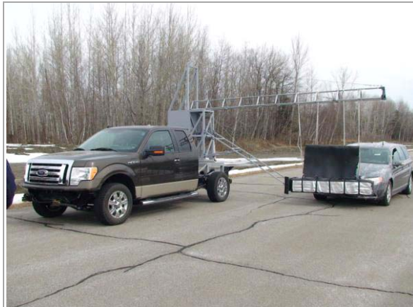
Figure 1. Mitigation braking test with mobile target
