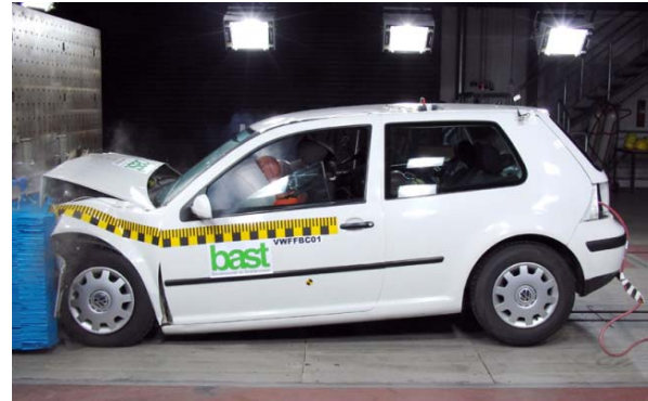
Figure 10: Small family car in full-width deformable barrier test
