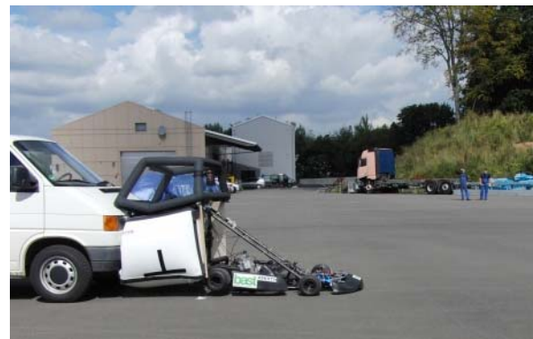
Figure 5: Test of the crashability of the ASSESS target with propulsion system carried out by BAST
