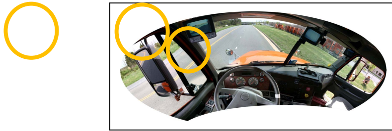
Figure 4. Placement of A-C/VIS monitors in truck cab.
