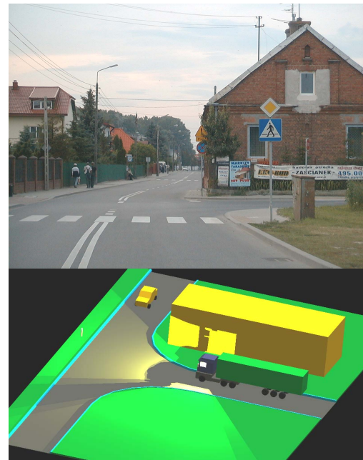
Fig. 6. The example above reflects the limitation of visibility on the crossing by the building which covers the part of the road for people arriving from the left and the diagram shows an example of this real situation.
