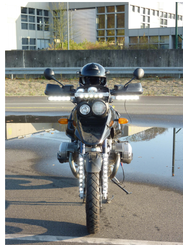
Figure 5: Test motorcycle with LED-DRL forming the T-arrangement
