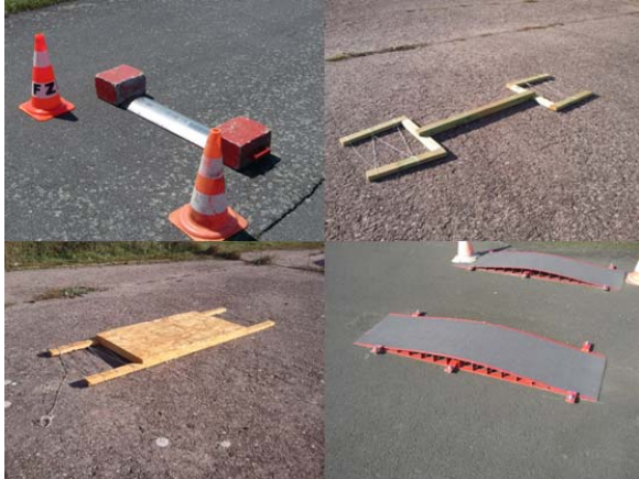
Figure 3: Obstacles: low speed bump, high cleat, duct cover, high cosine wave
