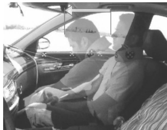
Figure 2: Longitudinal displacement of the occupant in the case of a braking maneuver with/without PRE-SAFE®
