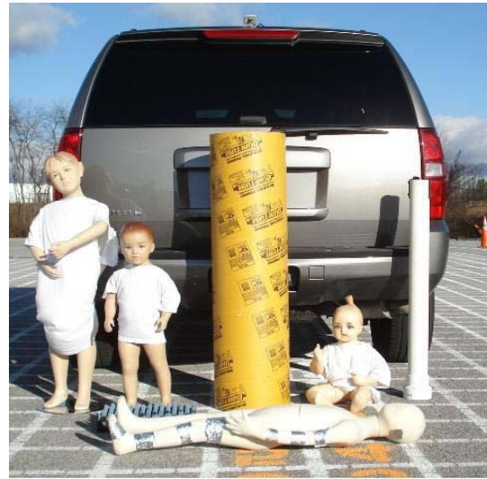
Figure 12. Test Objects used during testing (from left to right: Gen II 5 year old, Gen II 2 year old, Cardboard Cylinder, Gen II sitting child, PVC Pole, Gen I Prone 5 year old).
