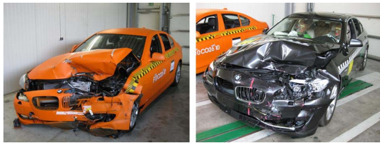
Figure 2. Different deformations resulting from the 64 km/h impact (orange) and the 40 km/h impact (black).
