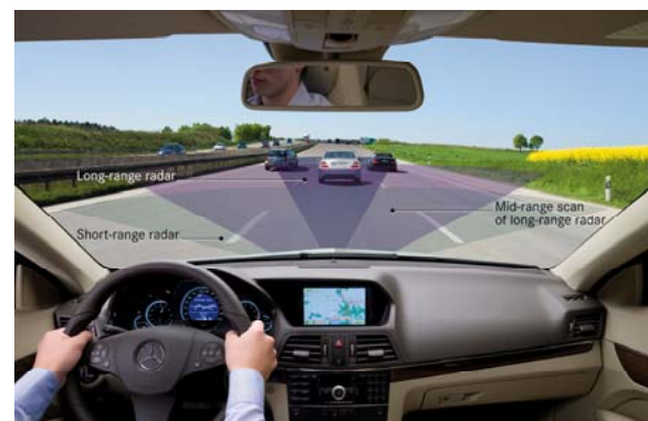
Figure 9: Area covered by short- and long-range radar
