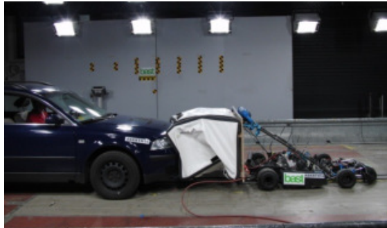
Figure 3. Test setup for crashability verification, early configuration.
