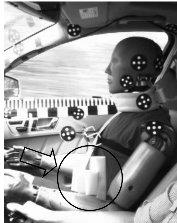
Figure 7: Foam layer on dummy for optimizing the occupant kinematics in the braking phase
