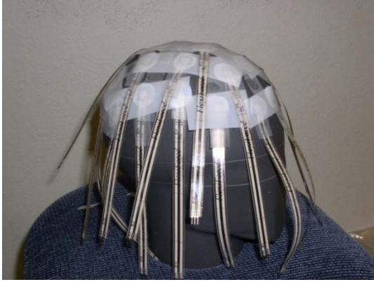
Figure 2. Fully instrumented headform for crown drops.
