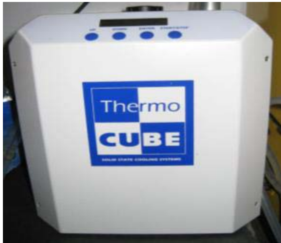
Figure 3. ACS prototype with DLS Swept Sensor™ technology and required chiller to maintain constant temperature
