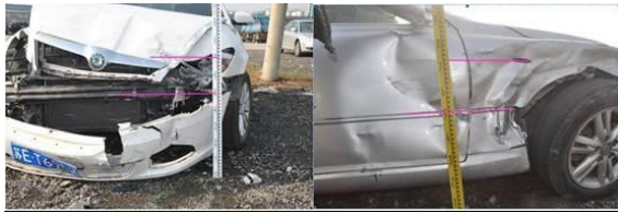
Figure 2. Vehicle deformation measurements
