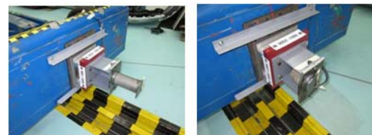
Figure 10. Dynamic test using the moving crash barrier
