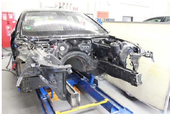
Figure 9. Car on the repair bench with disassembled front.
