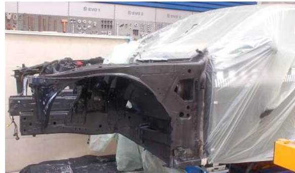
Figure 10. New components were attached with welding and adhesive.
