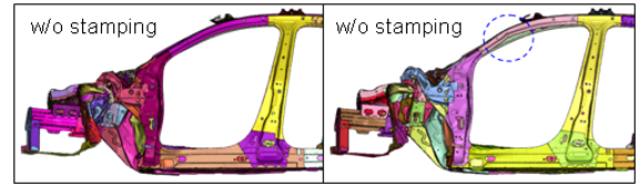
Figure11. Global deformation on BIW
