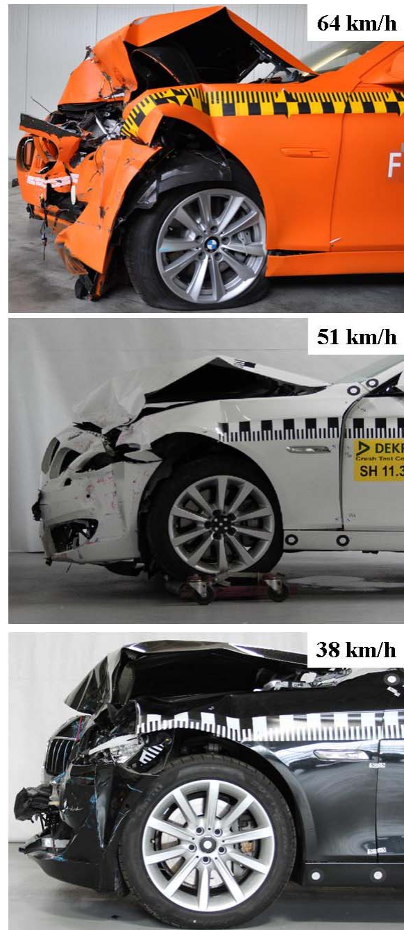
Figure 6. Comparison of the deformation of the front of the test vehicles (top down: 64, 51 and 38 km/h impact speed).
