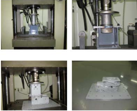
Figure 8. Static compression test of pre external inversion pipes and rectangular section crash box
