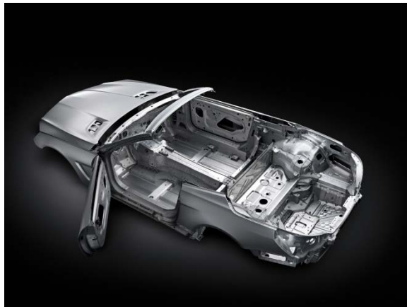
Figure3. SL lightweight bodyshell
