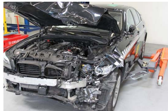
Figure 8. Deformations resulting from the 38 km/h impact.
