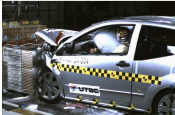
Figure 1. (PDB 60 km/h crash test).
