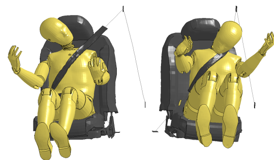
Figure 8: Comparison of the occupant kinematics for the 520mm passenger [Left] and 520mm driver side [Right] rigid pole offset impact at the final stage of the simulation (160ms). Front view.
