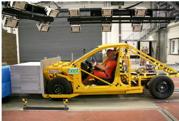
Figure 1 Side view of the reference vehicle with a PDB attached and Hybrid III dummies
