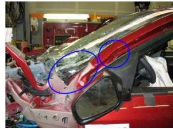
Figure12. Deformation view on BIW in the physical test
