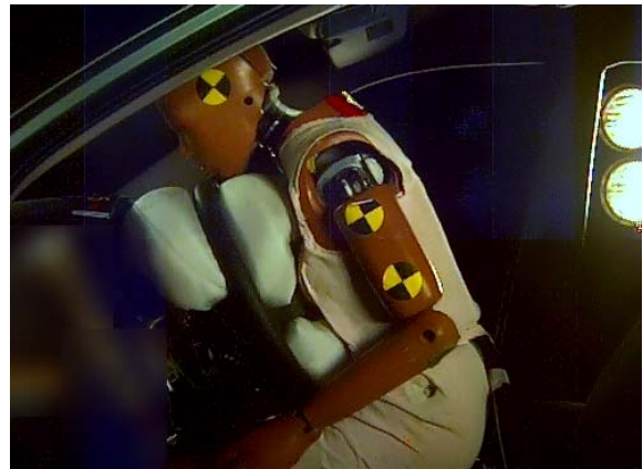
Figure 23. Confirmation OOP Test for NHTSA Position 2 at 15ms(Test 2 with Suggestion 1).
