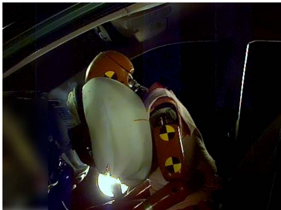
Figure 20. Confirmation OOP Test for NHTSA Position 1 at 15ms(Suggestion 1).
