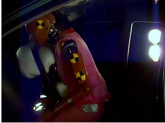
Figure 24. Confirmation OOP Test for NHTSA Position 2 at 15ms (Test 1 with Suggestion 2).
