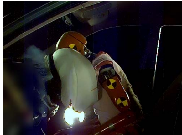
Figure 21. Confirmation OOP Test for NHTSA Position 1 at 15ms(Suggestion 2).
