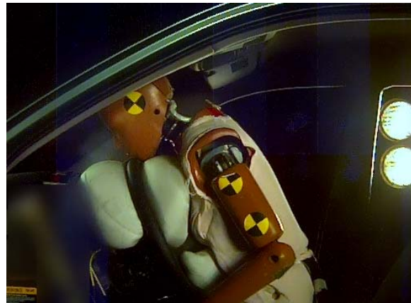
Figure 22. Confirmation OOP Test for NHTSA Position 2 at 15ms(Test 1 with Suggestion 1).
