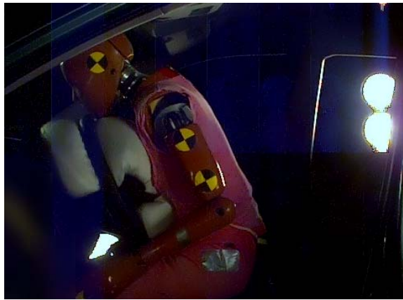
Figure 25. Confirmation OOP Test for NHTSA Position 2 at 15ms (Test 2 with Suggestion 2).
