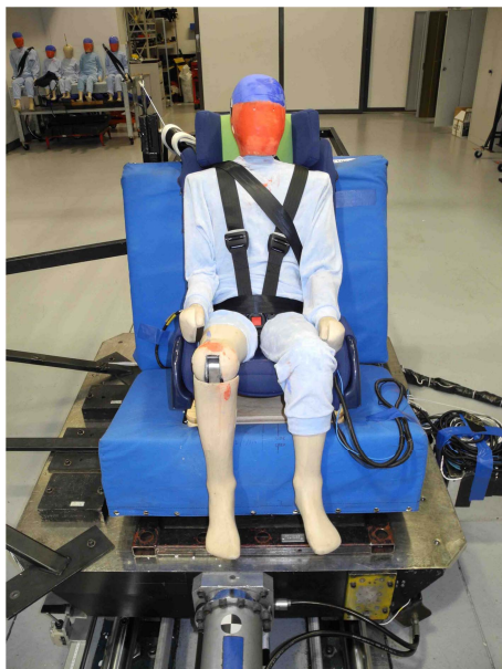
Figure 1: Sled, CRS and ATD frontal impact configuration.
