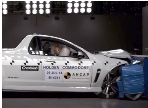
Figure 1. Research test vehicle impact with deformable barrier.
