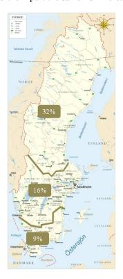
Figure 2. Fatal crash risk increase with non-studded tyres on non-ESC cars compared to studded tyres.
