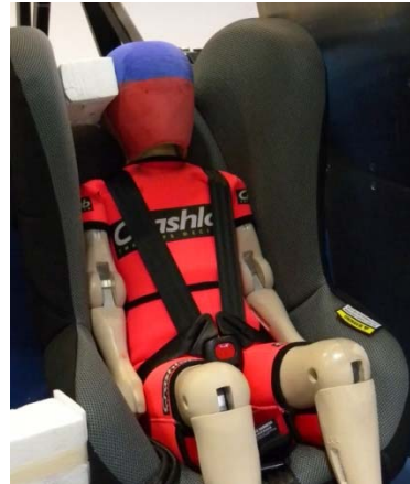
Typical side wing height change on FFCRS over CREP4-CREP5
