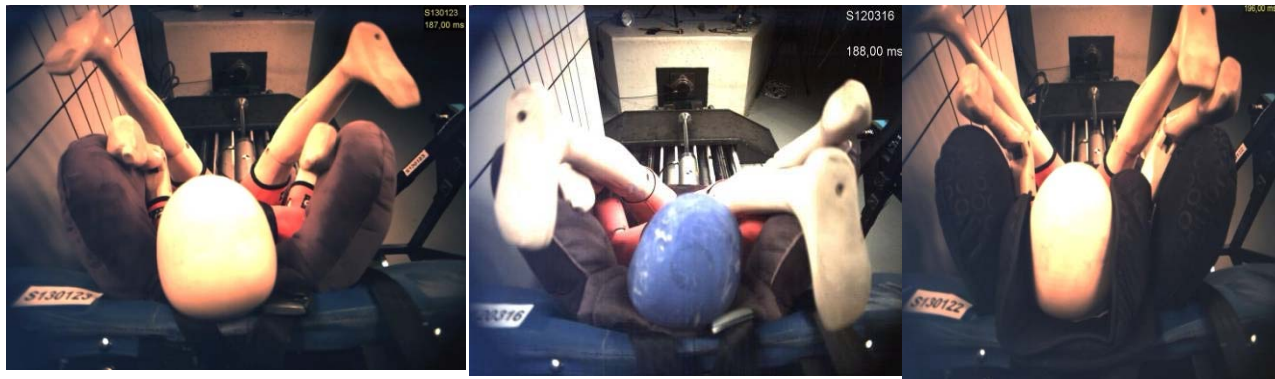
Head rotates overs 'dip' in seat back No structural support at top of back Head rest fails to support head Figure6. Poor support of dummy head in rebound during frontal impact
