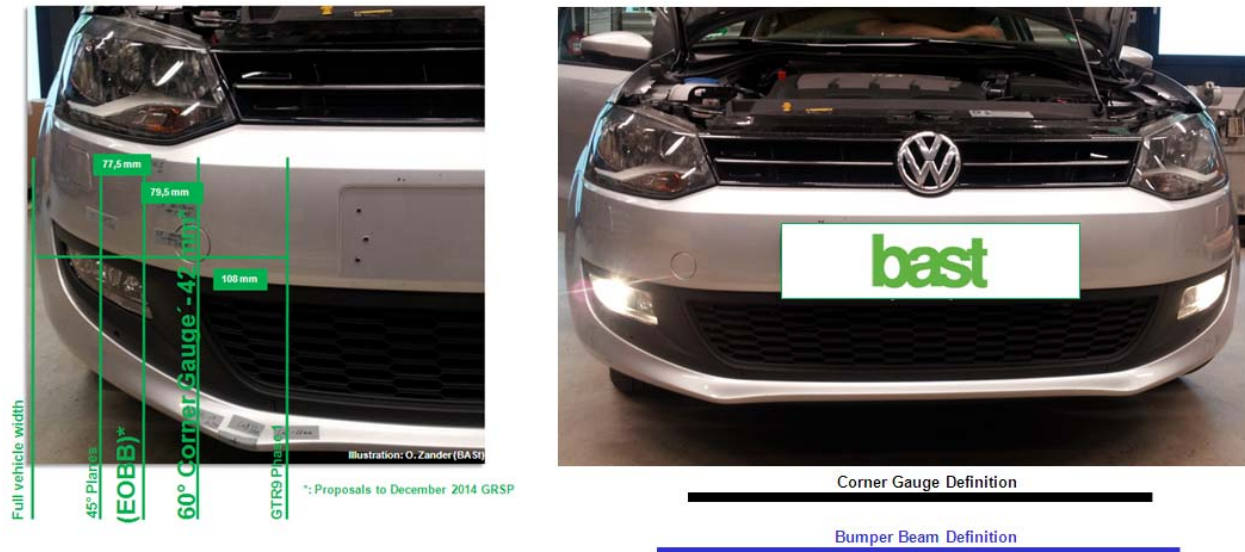
Figure 7. Comparison of different markup procedures and resulting test area widths.
