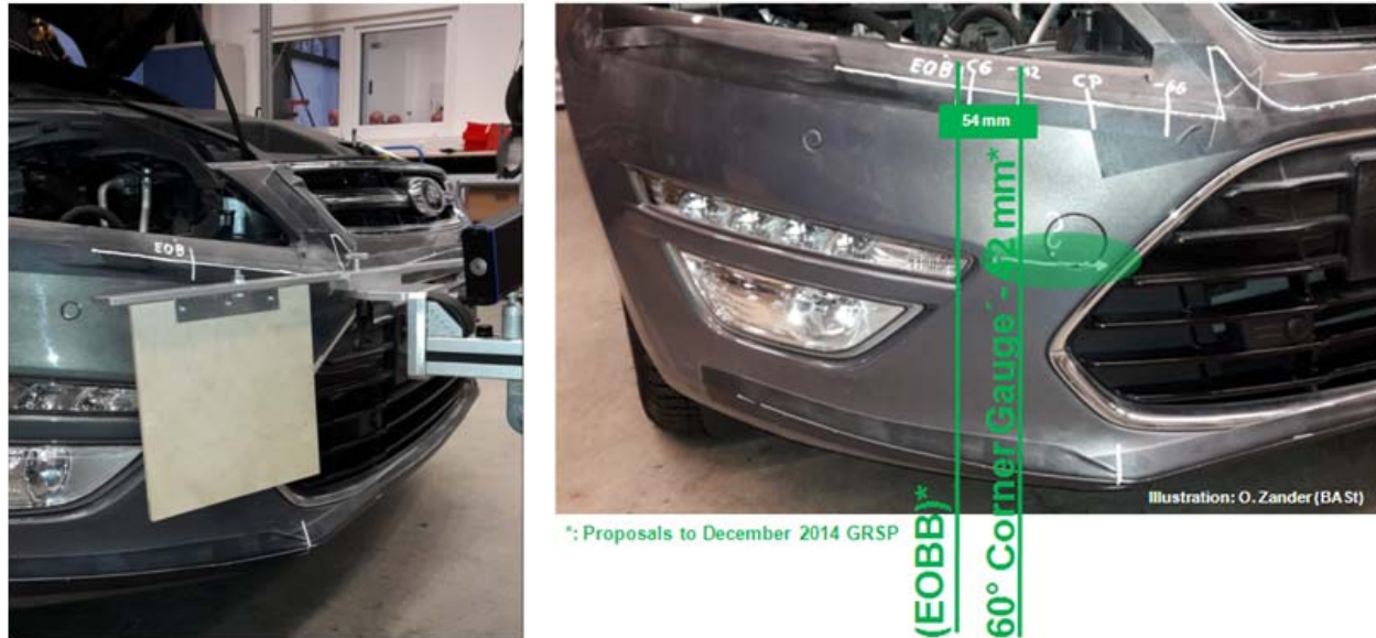
Figure 5. Corner point due to gauge contact with daytime running light intake.
