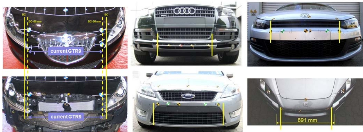
Figures 1a (left) and b (middle and right). Bumper test area according to GTR9 / UN-R 127 and its limitation by design means.
