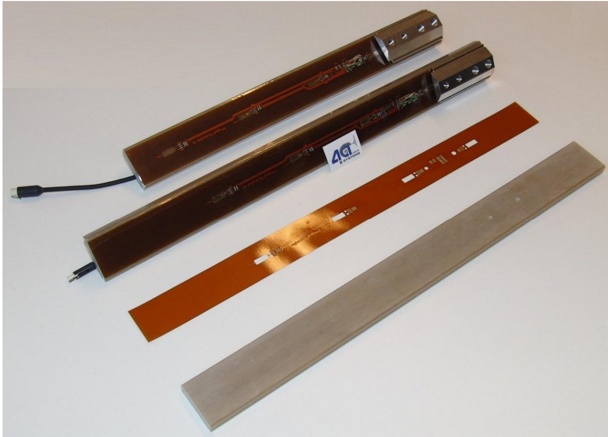
Figure 3: Final assembly of 4a femur bone core and 4a tibia bone core spare part, the PCB for a tibia as well as a tibia blank (from left to right) (photograph: 4a Engineering GmbH)
