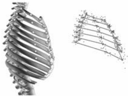
Figure 1: Landmark points shown for geometric model development (left) and superimposed landmark points from CT scans (right).
