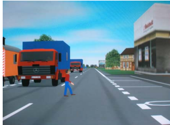
Fig. 2: Critical situation simulated by the DaimlerChrysler Berlin Driving Simulator: child crossing an urban street
