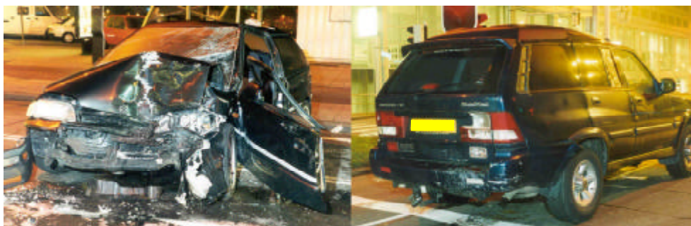
Figure 3. The front of a small passenger car that drove into the back of a SUV.
