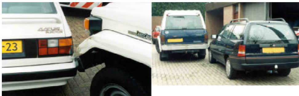
Figure 1. Difference in the height of the bumpers.
