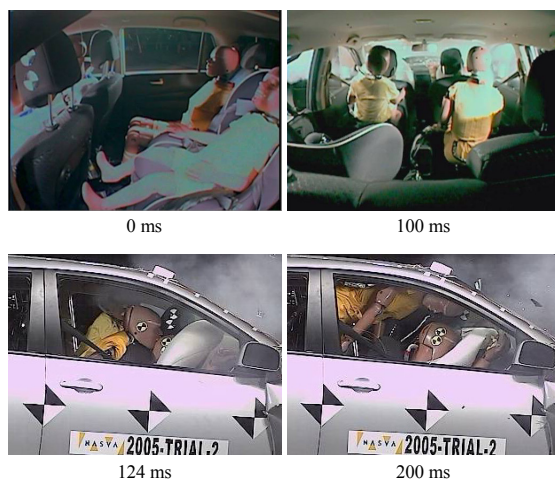
Figure 7. Kinematics of unbelted Hybrid III AF05 in rear seat (test 2).
