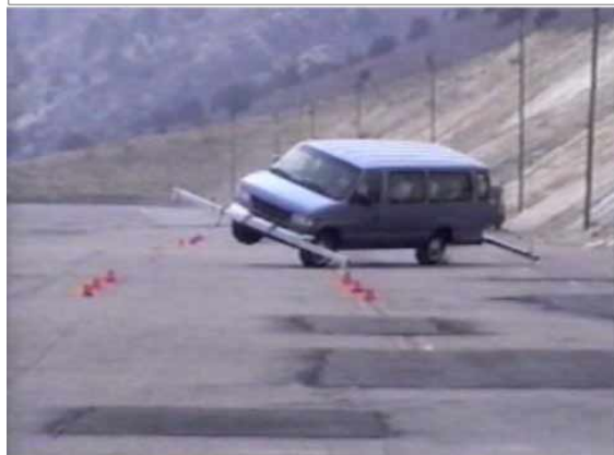
Figure 11. Test 4 – NHTSA Fishhook with unmodified vehicle and single rear wheels.
