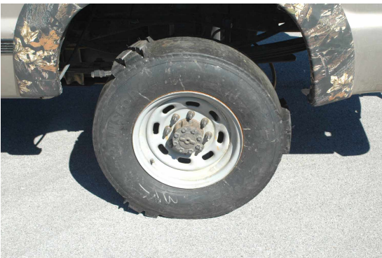
Figure 4. Prepared tire with vulcanized lumps.
