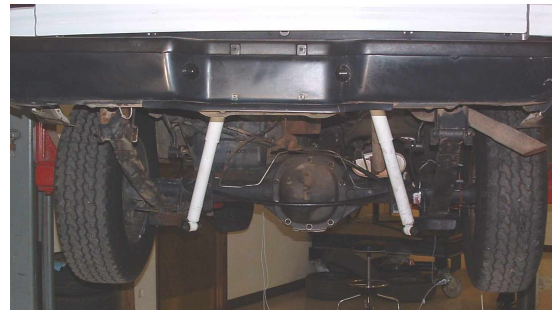
Figure 5. Hotchkiss rear suspension system showing shock placement.
