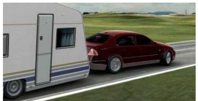
Figure 11. ESP® function “Trailer Sway Mitigation” to counteract sway movement induced by external excitation (e.g. side wind, road bump)
