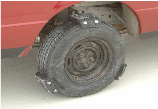
Figure 3. Prepared tire with bolted lumps.
