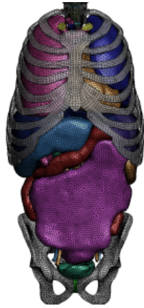
Figure 2. Skeletal structure and internal organs of torso model.
