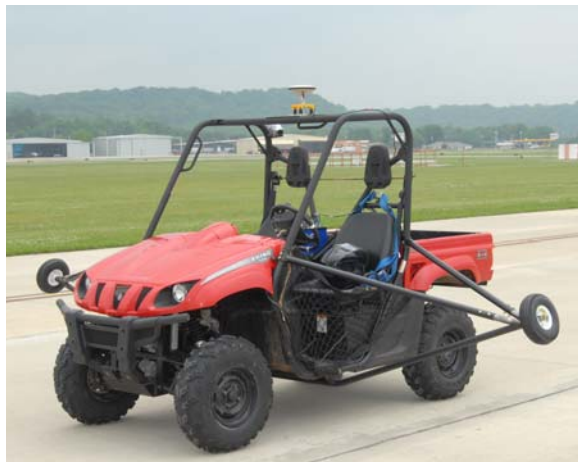
Figure 2. Test vehicle as prepared for testing (Yamaha Rhino 450).
