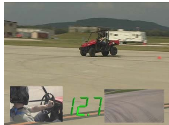
Figure 9. Frame capture from vehicle testing showing onset of loss of directional stability characterized by a lifting of the inside rear tire (the green is speed in mph).
