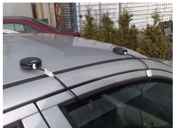
Figure 1. The reference GPS sensors in set-up designed for verification of statistical robustness of the positioning subsystem of the in-vehicle eCall unit.
