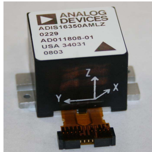
Figure 3. 6-DOF reference inertial measurement unit ADIS16350
