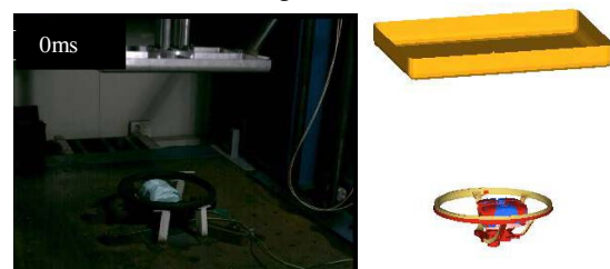
Figure 9. Initial stage of Drop Tower Test with folded bag
