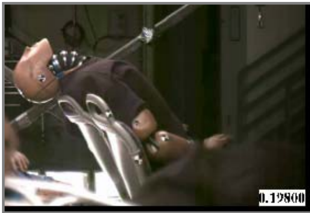
Figure 23. Crash Condition 20 mph Bus – 0 mph Bus Rear Impact (5 th , 50 th and 95 th percentile Passenger Kinematics).
