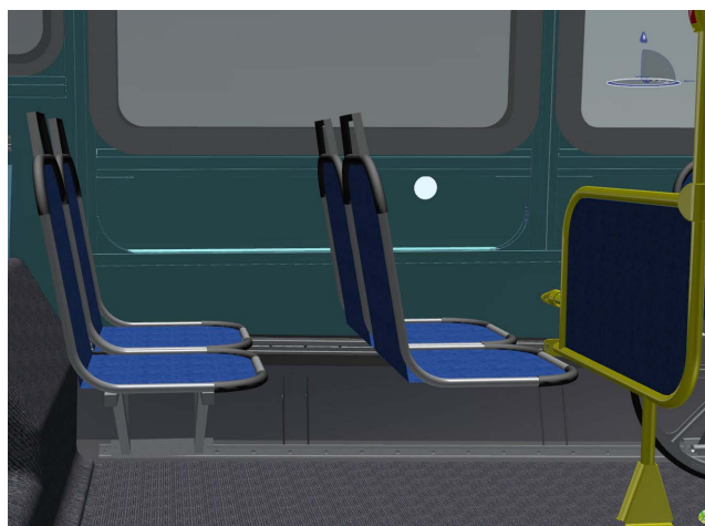
Figure 6. Seat-to-Seat Configuration (left), and Seat-to-Divider Configuration (right).
