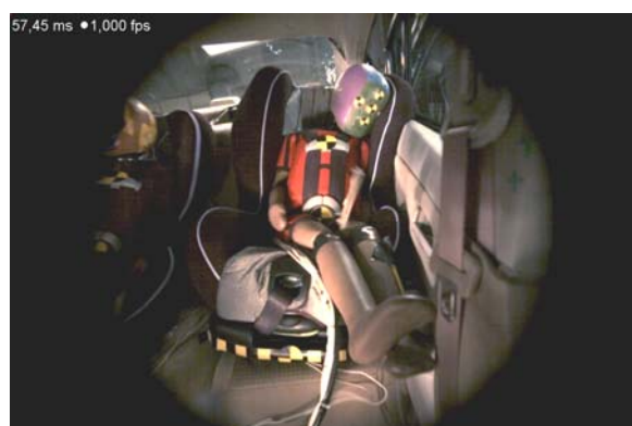
Figure 20. Near-side Dummy (Test #v06635, Sentra); Example of CRS Base Rotation and Angular Door Intrusion.
