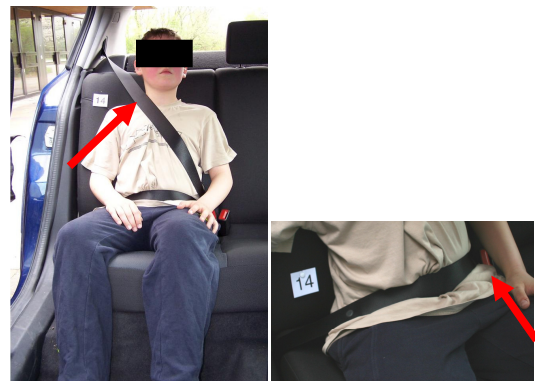
Figure 1. 10 year old boy (body size 144.2 cm, body weight 41.6 kg) in an Opel Astra (model year 2003) without child restraint system. Arrows indicate critical positions of the safety belt.
