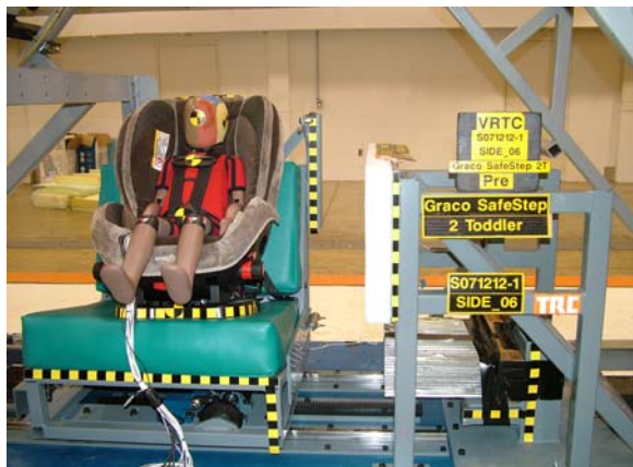
Figure 2. NHTSA’s Side Impact Sled Buck Set-up.
