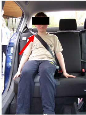
Figure 2. 10 year old boy (body size 144.2 cm, body weight 41.6 kg) in an Opel Astra (model year 2003) with child restraint system.
