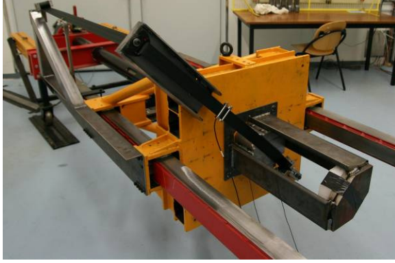
Figure 7. Sled crash setup used to test the belt force actuator during impact.
