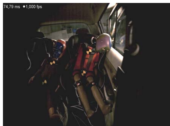
Figure 29. Q3s Dummy Head Contact, Maxi-Cosi Priori in Versa #v06637.
