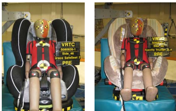
Figure 11. Examples of Wing Designs (Graco SafeSeat Step2 [left] and Evenflo Triumph [right]).
