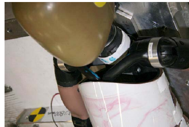
Figure 13. Touched sign of Q3 Dummy clavicles and spine after the test of 5-point harness CRSs
