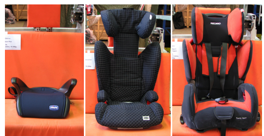
Figure 7: Three typical CRS. From left to right: no-back booster seat (group II/III), high-back booster seat (group II/III) and combination seat (group I/II/III).
