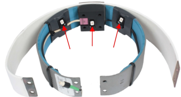
Figure 4. RibEye LEDs installed on WorldSID rib [8]
