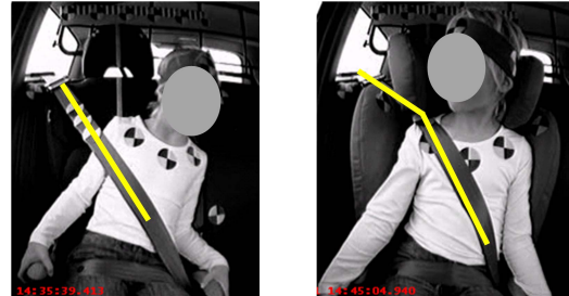
Figure 10. Lateral inboard motion of a child during a steering maneuver, using booster cushion (left) and booster seat (right), (Bohman et al. 2011b)
