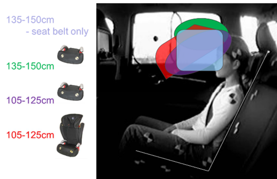
Figure 4. Schematic plot representing trajectories for forehead targets for child volunteers (Stockman et al. 2013a).
