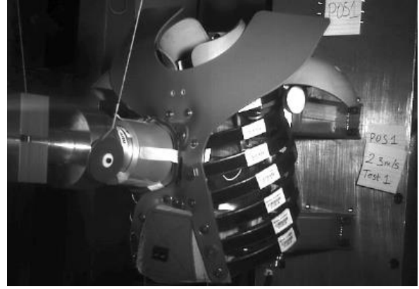
Figure 9. Local deflection of bib in the area of an offset pendulum impact
