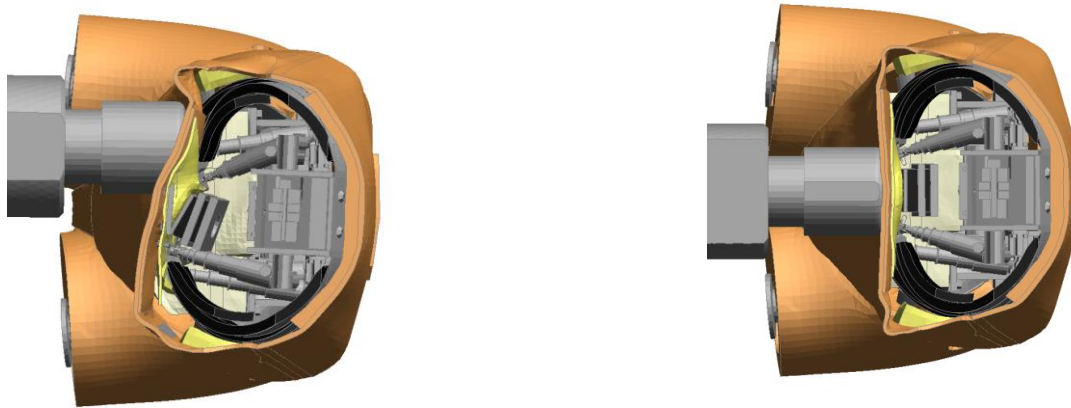
Figure 11. Local deflection of bib in the area of central and offset pendulum impacts
