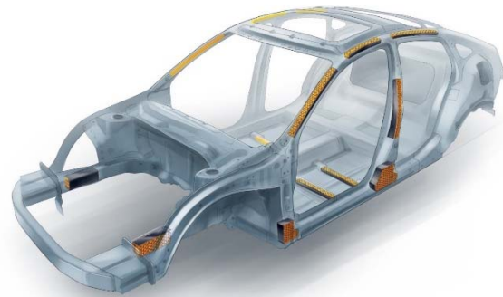
Figure 5. Few BIW reinforcements in typical automobile. Adapted from [11].
