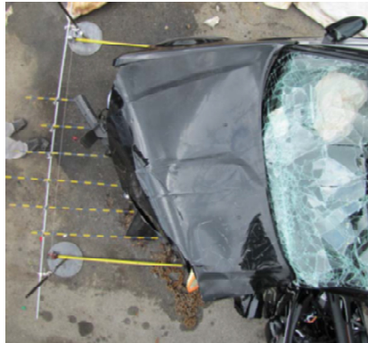
Figure 20. Post-crash vehicle static crush measurements
