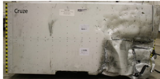
Figure 18. Post-crash photo of the OMDB deformation
