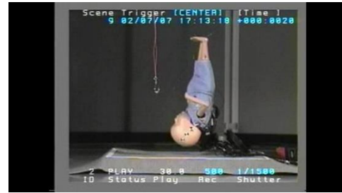
Figure 2: Vertex Drop Test Setup
