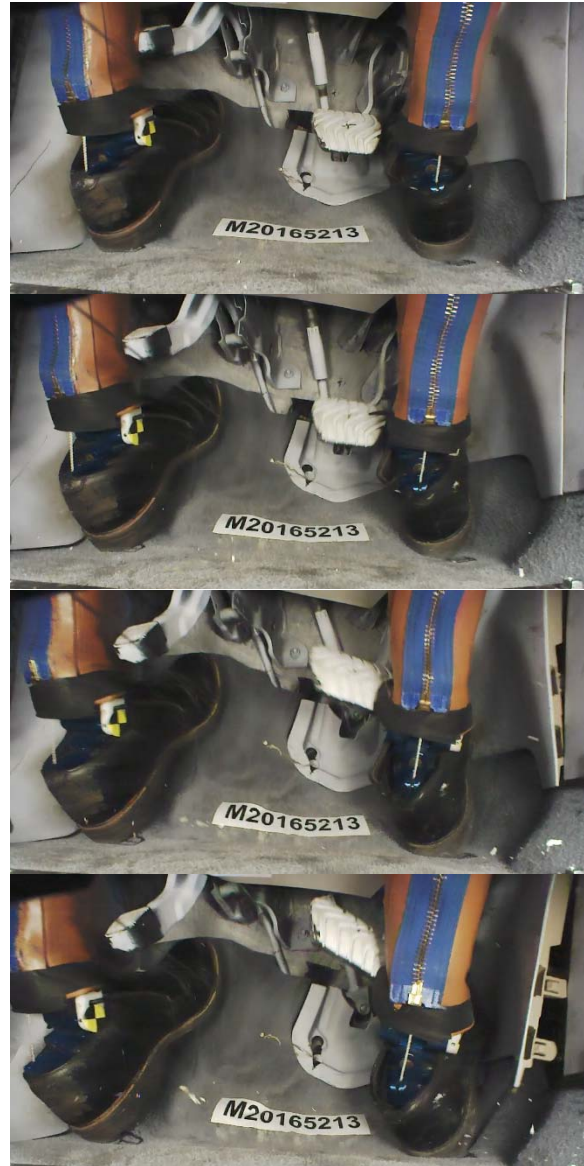
Figure 9: Still frames extracted from test 9574 at 0.030, 0.035, 0.040 and 0.045sec after the impact.
