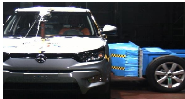
Figure 3. KNCAP side impact test configuration
