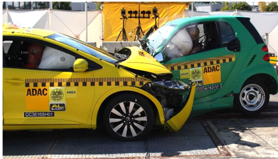
Figure 5: Car to car impact with THOR dummy
