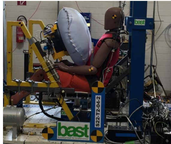
Figure 4: THOR R&R sled testing
