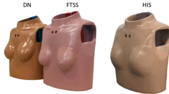
Figure 1. Comparison of Harmonized (HIS) Chest Jacket to the DN and FTSS brand for the Hybrid III 5 th Percentile Female Dummy [2]
