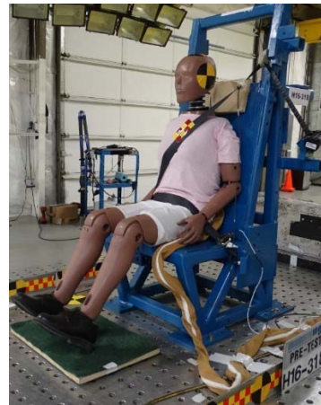
Figure 4. Controlled sled test set-up
