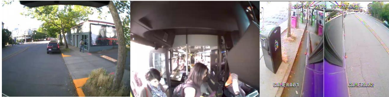
Figure 3. Left to Right - Images captured by Rosco Dual-Vision: Channel 1 forward-facing, Channel 2 interior rear-facing, Channel 3 split screen left and right external side cameras.
