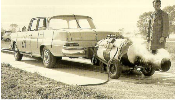
figure 1: In the late 1950s, vehicle crash testing was conducted using a rocket propelled by hot steam [Daimler archive]
