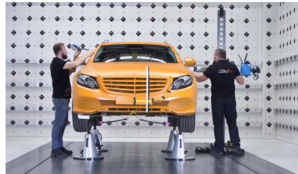
figure 12: 3D spot measurement [Daimler]
