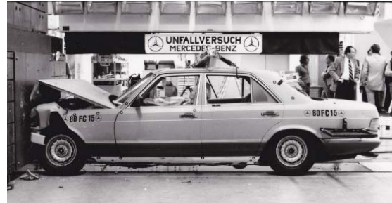
figure 3: 1980: S-Class W126 in a full frontal crash test in the Sindelfingen crash test facility [Daimler archive]
