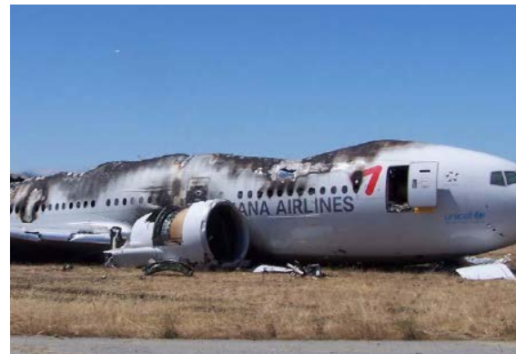
Figure 4: Fire damage to the fuselage of flight 214.
