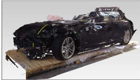
Figure 2. Image depicting linked 3D scans of the passenger vehicle used for measurements.
