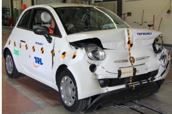
Figure 3. Test 2: Post-test photo, 45-degree view, after 50 km/h, full-width, rigid barrier frontal impact test according to R137
