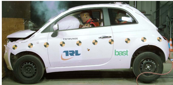
Figure 8. Test 6: Test photo at maximum pitch angle of low-speed (35 km/h), full-width, rigid barrier frontal impact test
