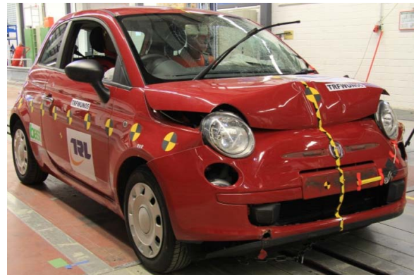
Figure 4. Test 5: Post-test photo, 45-degree view, after low-speed (35 km/h), full-width, rigid barrier frontal impact test
