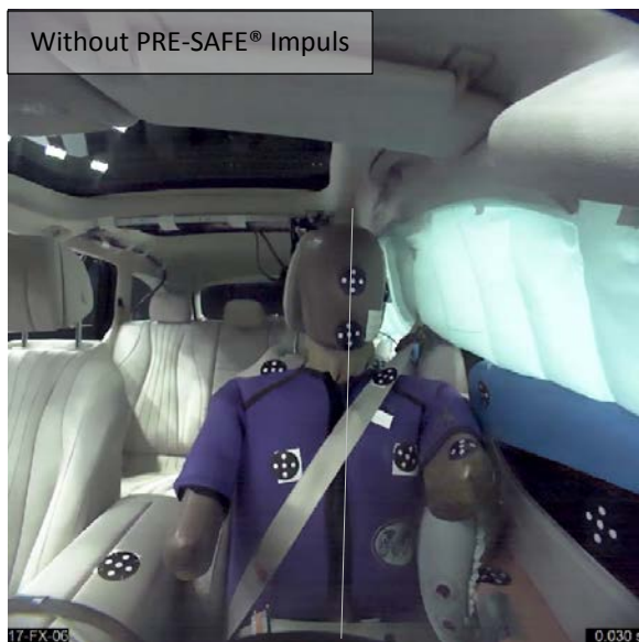
Figure 14: Dummyposition @ 30ms without PRE-SAFE® Impuls
