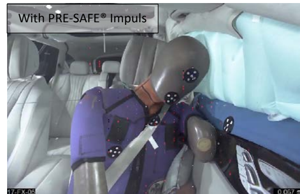
Figure 15: Dummyposition @ 67ms with PRE-SAFE® Impuls
