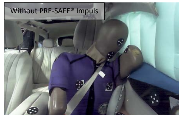
Figure 16: Dummyposition @ 67ms without PRE-SAFE® Impuls
