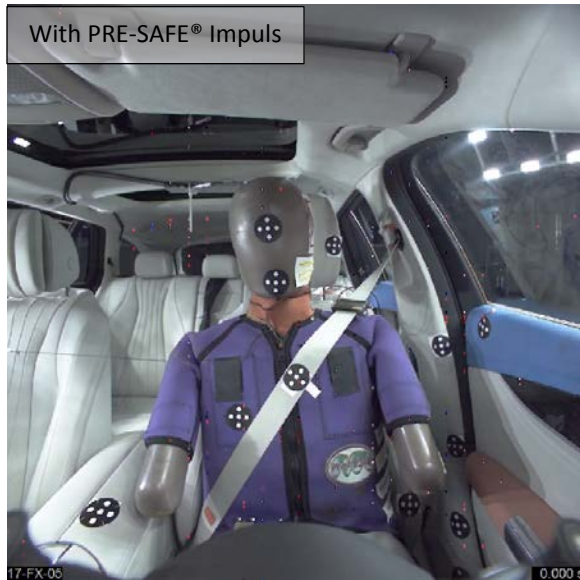
Figure 9: Dummyposition @ 0ms with PRE-SAFE® Impuls
