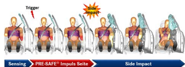
Figure 3: Occupant interaction due to PRE-SAFE Impulse activation
