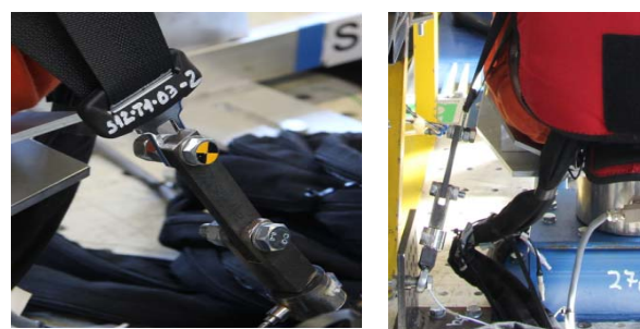
Figure 3. Generic buckle with uni-axial load cell
