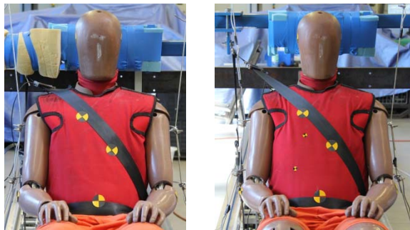
Figure 12. Variation of belt routing on chest due to different D-ring position (left: D1; right D2)
