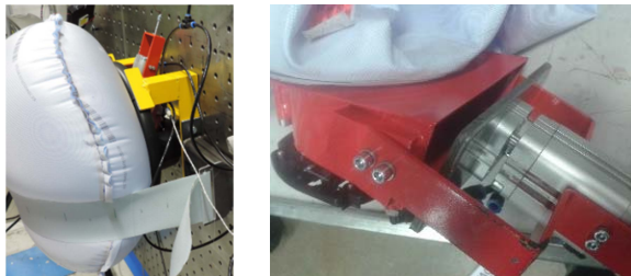
Figure 10. Ventilation mechanism, steering wheel support and external strap.
