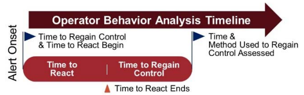
Figure 3. Sequence of Dependent Variables pertaining to driver behavior adapted from previous test track studies.
