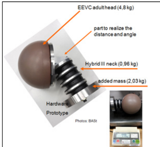
Figure 8: APROSYS head neck impactor HNI.
