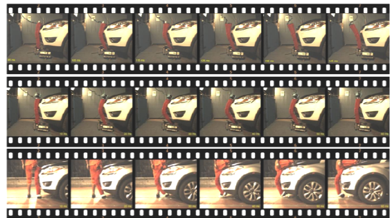
Figure 13: Correlation of impact kinematics between FlexPLI, FlexPLI-UBM and FlexPLI-HII (Zander et al., 2011).
