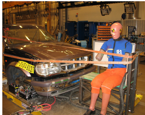
Figure 10: Sled test setup with ES-2-dummy and vehicle buck (Fredriksson et al., 2007).
