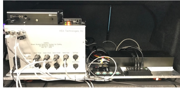
Figure 9. DADSS X2 Instrumentation located in the vehicle trunk
