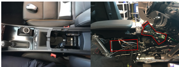
Figure 8. 4 th Generation touch-based sensor integrated in the DADSS X2 research vehicle center stack
