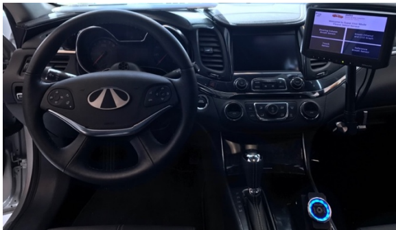
Figure 6. DADSS X2 interior with steering column breath-based sensor (top left), touch-based sensor (bottom right), and control monitor (top left)
