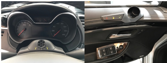
Figure 7. 3 rd Generation breath-based sensor integrated into DADSS X2 research vehicle steering column (left) and driver door panel (right)
