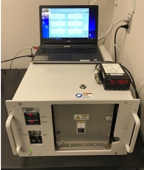
Figure 13. FTIR used for verification of the breath-based SCDs
