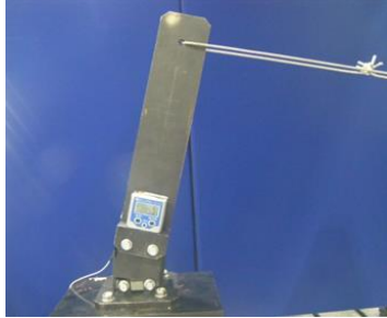
Figure 5. Lumbar spine flex joint bending test
