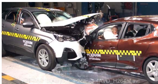
Figure 16 : C2C Peugeot 3008 vs Renault CLIO (performed by UTAC)
