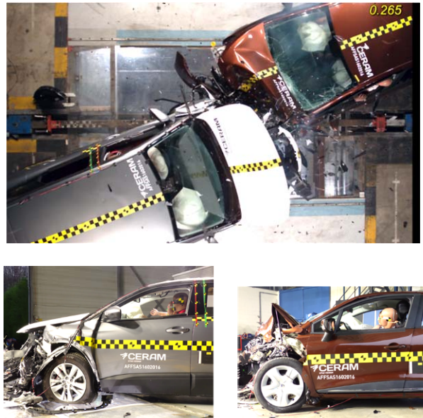
Figure 25 : Peugeot 3008 & Renault CLIO after C2C test (UTAC)
